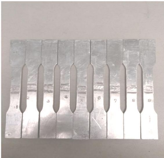
Fig. 4 Tensile test specimens as per ASTM E8 standard
