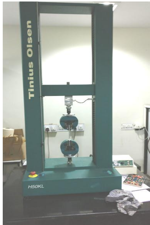
Fig. 5 Tensile testing machine TINUS OLSEN /L SERIES H50KL at CHARUSAT
