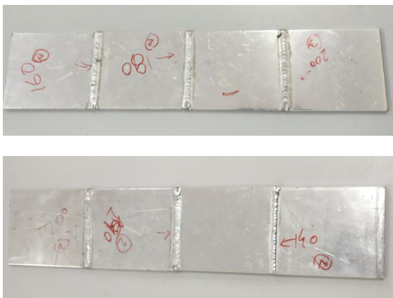
Fig. 1 The rough specimen used for estimating the required welding current.
