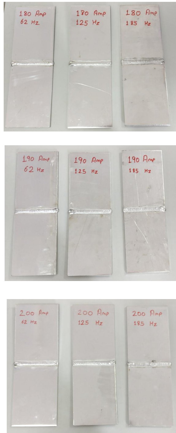
Fig. 2 Weld specimens prepared for different combinations of peak current and frequency as per table 2.
